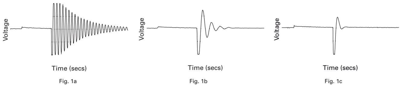
Diagrams of the waveform of the non-invasive neurostimulation device showing a) no skin contact, b) high-impedance skin contact, and c) low-impedance skin contact. The waveform dynamically adjusts in relation to changes in the skin. This allows localisation of sites of low impedance which are then specifically targeted. Conductive gel is not required.
