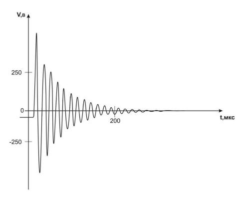
Fig. 1. Electrode voltage waveform before the electrode is put on skin
