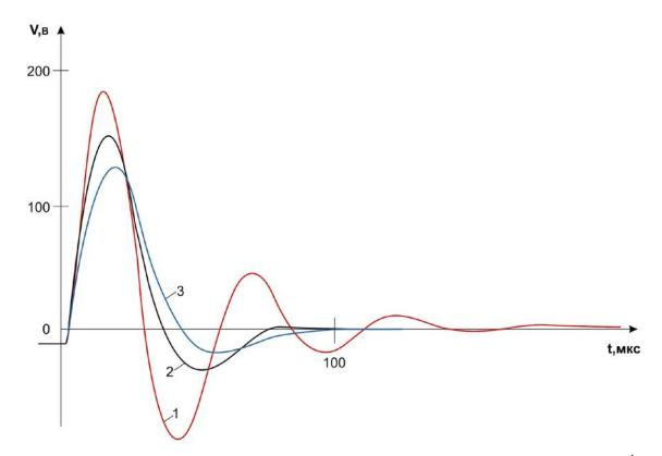
Fig.2 Variants of voltage waveforms in SCENAR stimulation.  $1 - \text{signal in } 0.22 \text{ sec } (13^{\text{th}} \text{ pulse}); 2 - \text{signal in } 1 \text{ sec } (60^{\text{th}} \text{ pulse}); 3 - \text{signal in } 10 \text{ sec } (600^{\text{th}} \text{ pulse}).$
